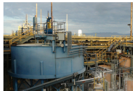
Sulf-IX™ plant removes calcium and sulphate hardness from wastewater for discharge.
