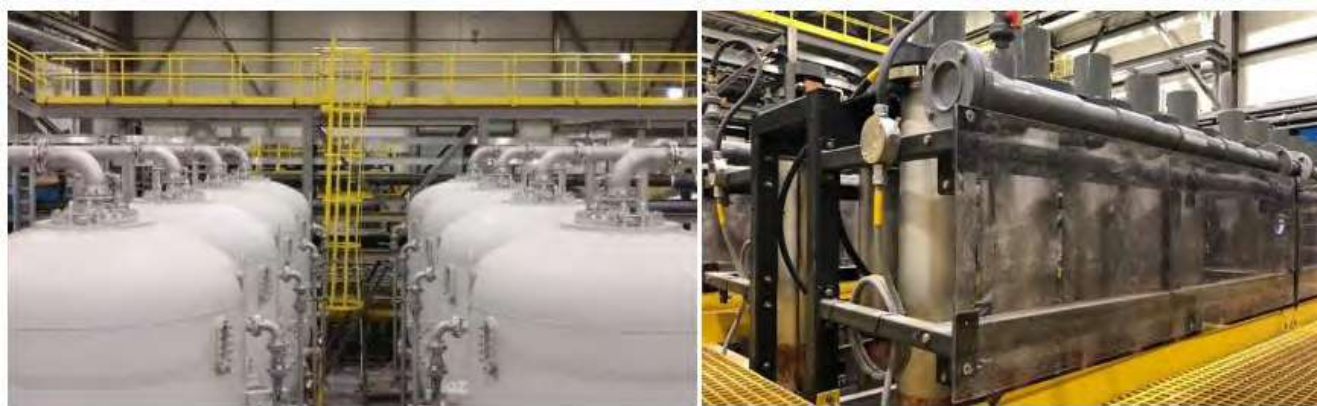
Figure 2: Kemess Selen-IX™ Plant with IX and ERC Circuits
